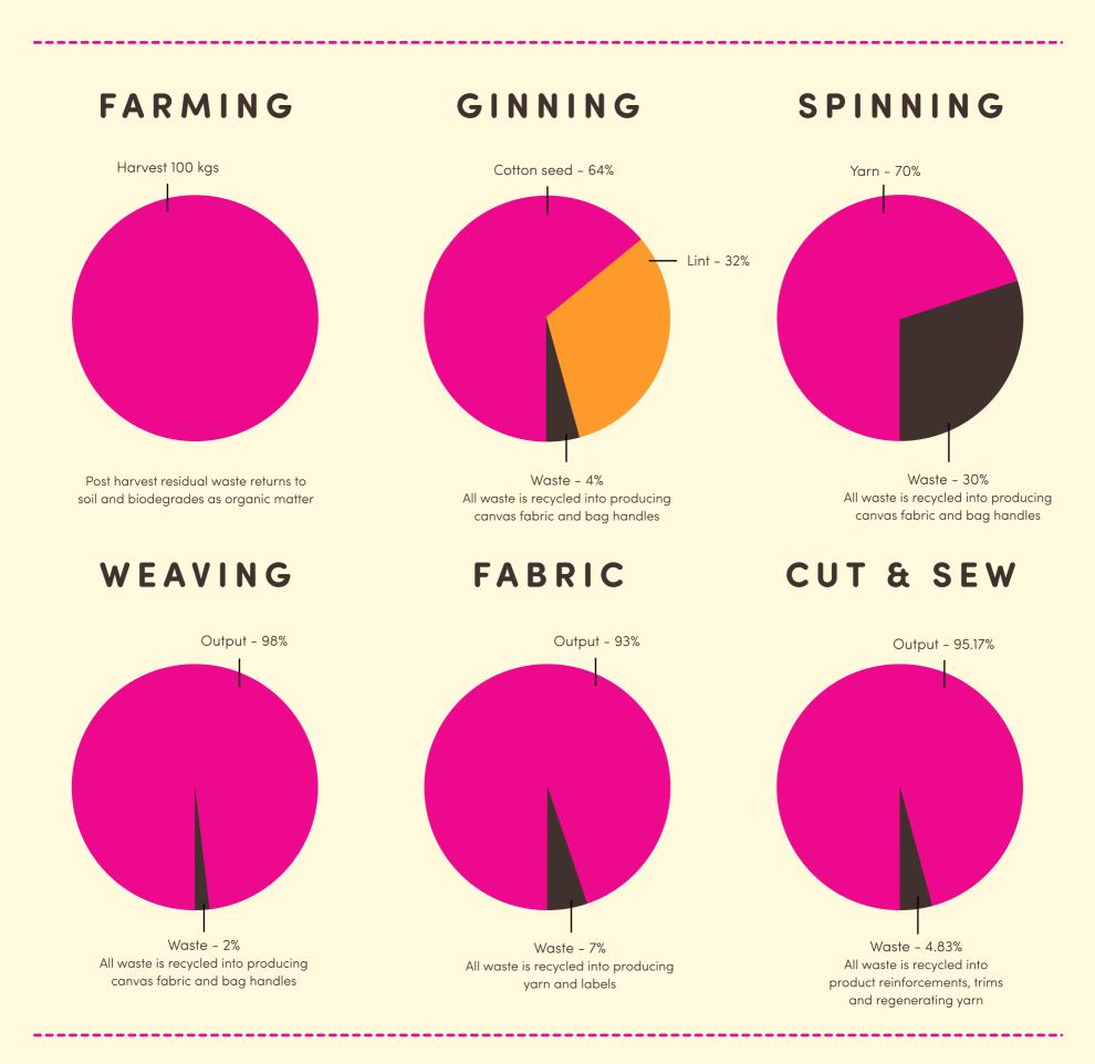
Different stages of a bag making process and its waste generation
